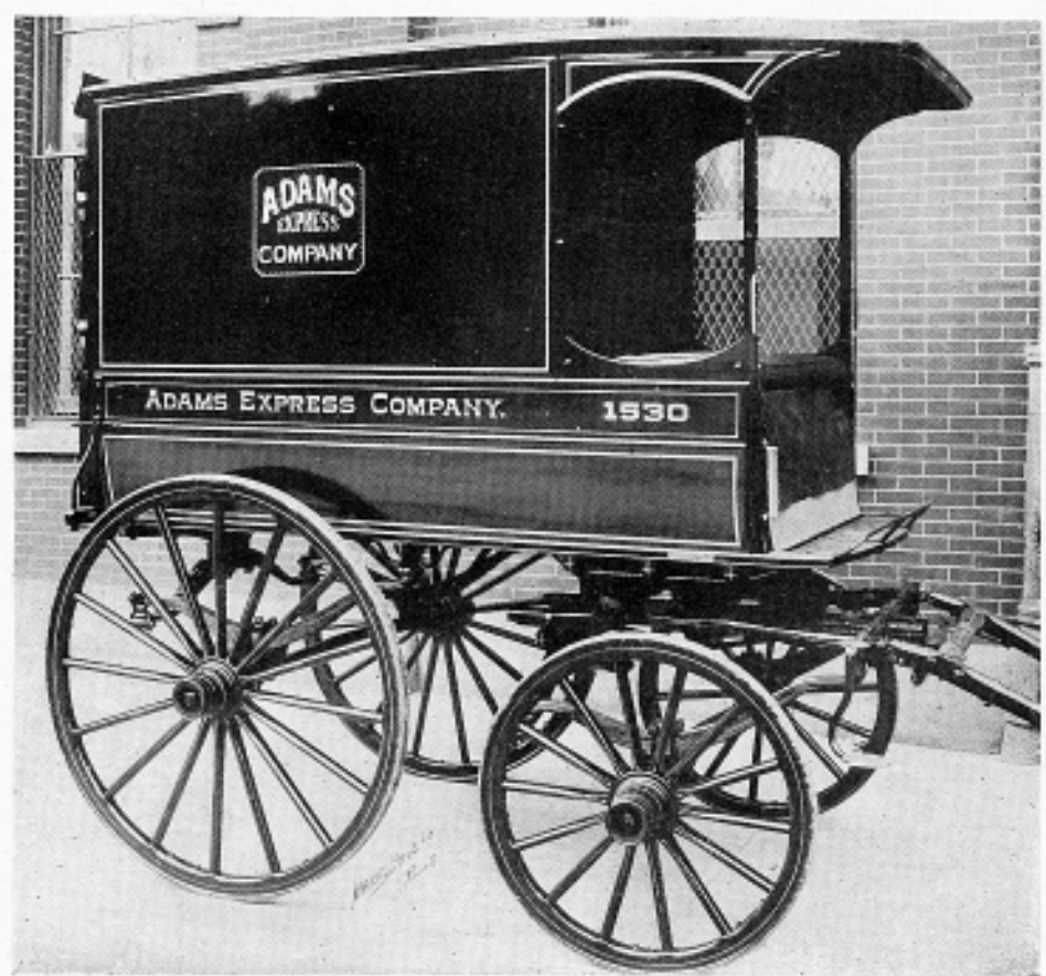
PLATE No. 1507. DELIVERY WAGON, WITH SOLID RUBBER TIRES. BUILT BY H. KAISER & CO., PHILADELPHIA, PA.
